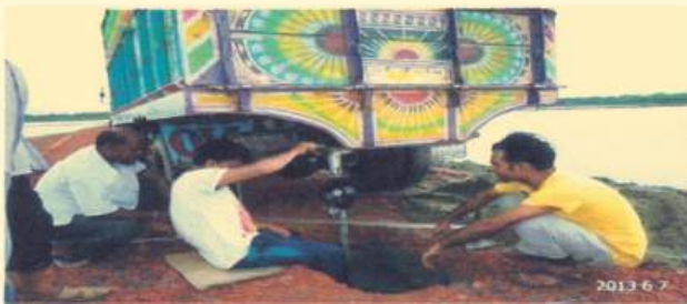
Fig: Conducting field CBR test during 1st monitoring
