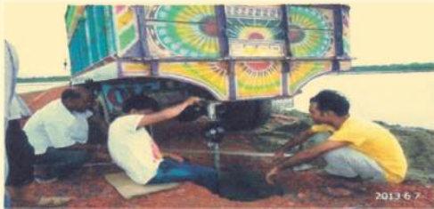
Fig: Conducting field CBR test during 1st monitoring
