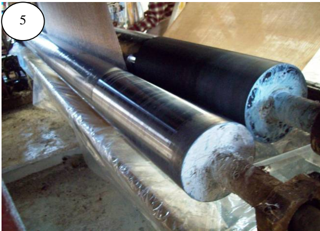
SQUEEZING OFF NR DIPPED FABRIC
