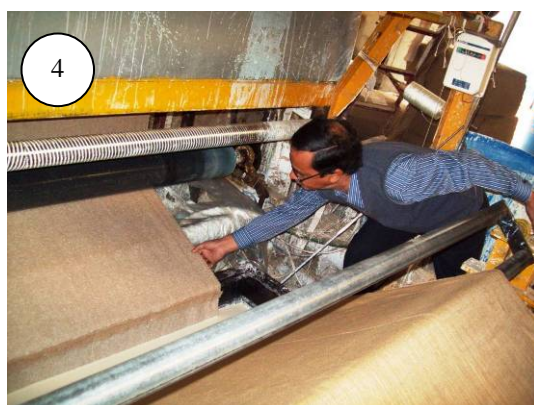
CONTINUOUS DRAWING OF JUTE FABRIC THROUGH COMPOUNDED NR LATEX
