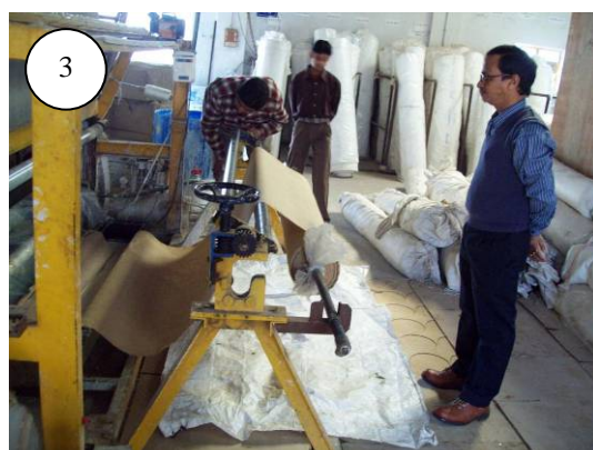
CONTINUOUS DRAWING OF JUTE FABRIC THROUGH COMPOUNDED NR LATEX
