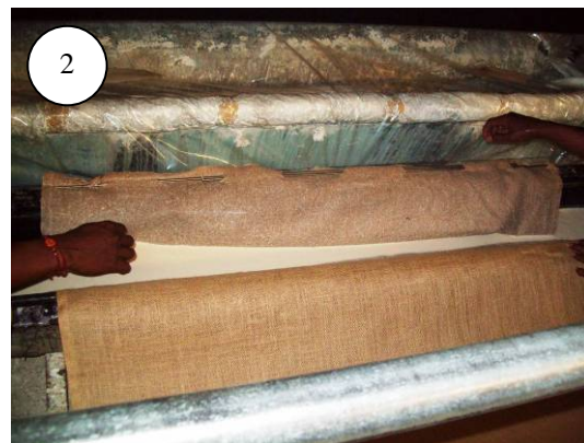
JUTE FABRIC DIPPING IN NR LATEX
