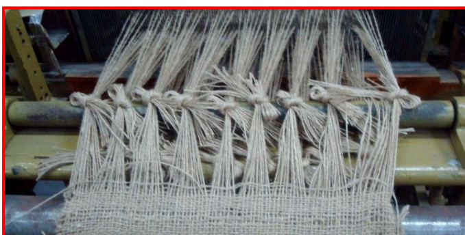
Fig 37-b : Gaiting of warp for Top fabric
