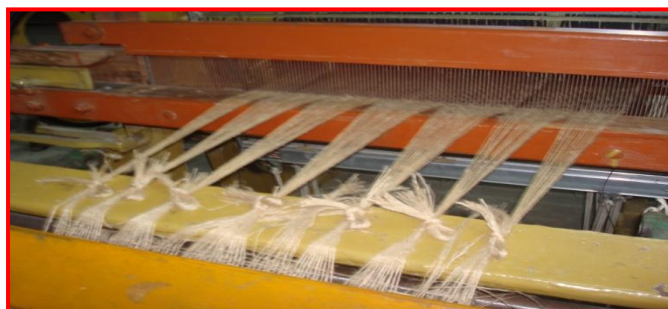
Fig 29 : Gaiting of beam
