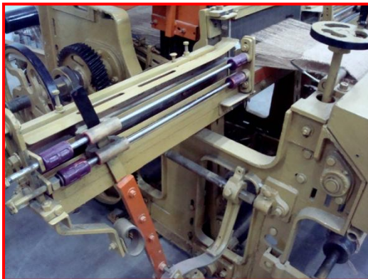
Fig 9-a : Shuttle Box (Left)
