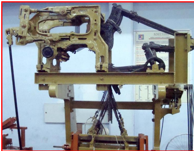
Fig 30 : Modified Heavy Duty Dobby
