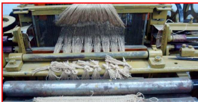
Fig 37-a : Gaiting of warp for bottom fabric
