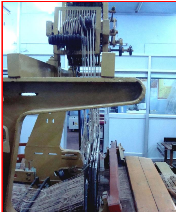
Fig 23 : Fitting of heald frames
