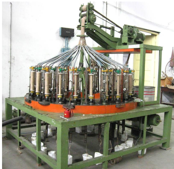
Fig. 6.2.13 Present actual view of the jute braiding machine (after modification)
