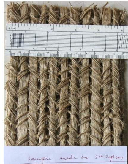
Fig. 7.1.3. Braided Jute sleeve combining 24 jute tape as axial material and two 8 lb/ spynkle jute yarns in each yarn carrier
