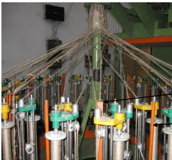
Fig. 6.2.9. Braiding machine mounted with rigid and flexible guides for axial materials
