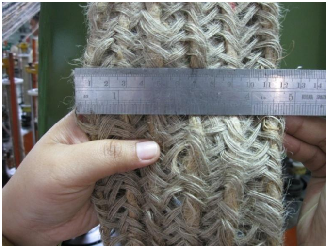
Fig. 7.1.2. Braided jute sleeve combining 12 jute roves as axial material and four 8 lb/ spynkle jute yarns in each yarn carrier
