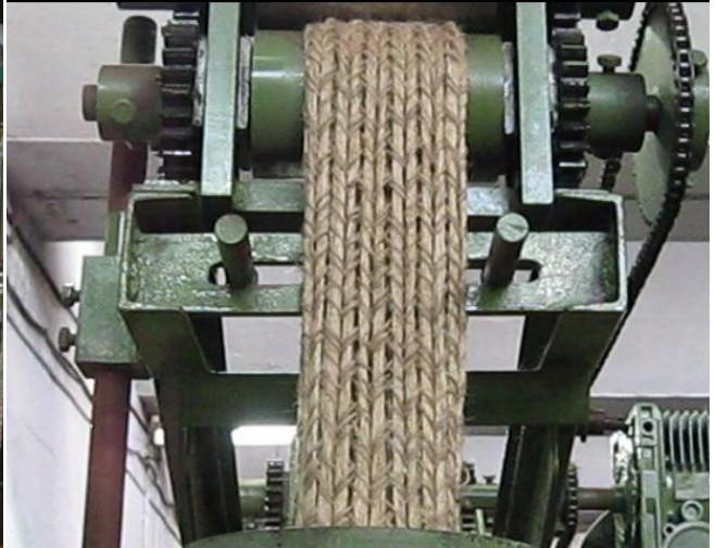
Fig. 6.2.12. Appearance of braided sleeve during braiding with 24 flexible guides for axial materials
