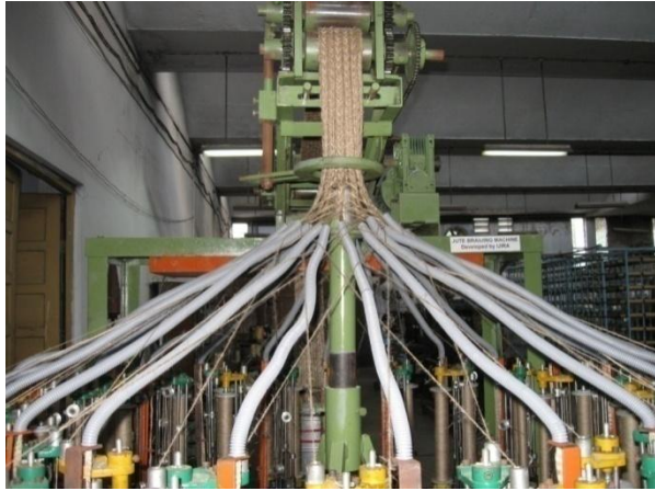
Fig. 7.2.1. Braiding with 24 jute axial tape utilizing 24 flexible plastic pipes as their guides
