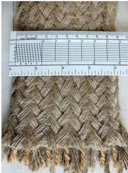
Fig. 16 Braided Vertical Drain: made of jute braided sheath and coir yarn core
