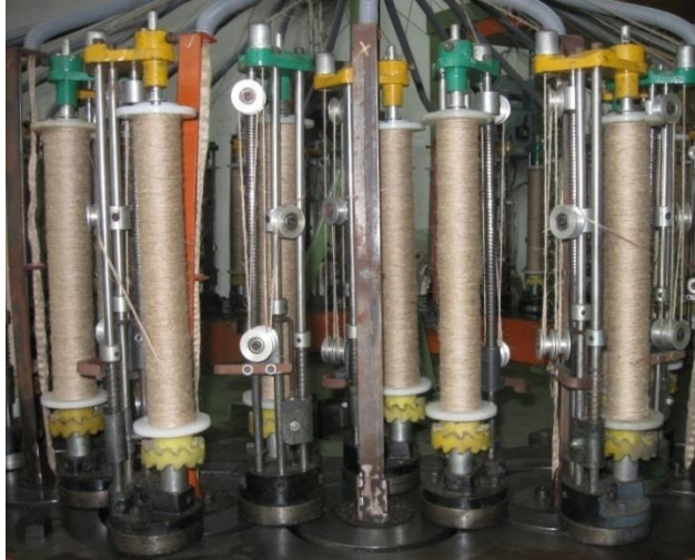
Fig. 6.2.11. Braiding machine mounted with all 24 flexible guides for axial materials
