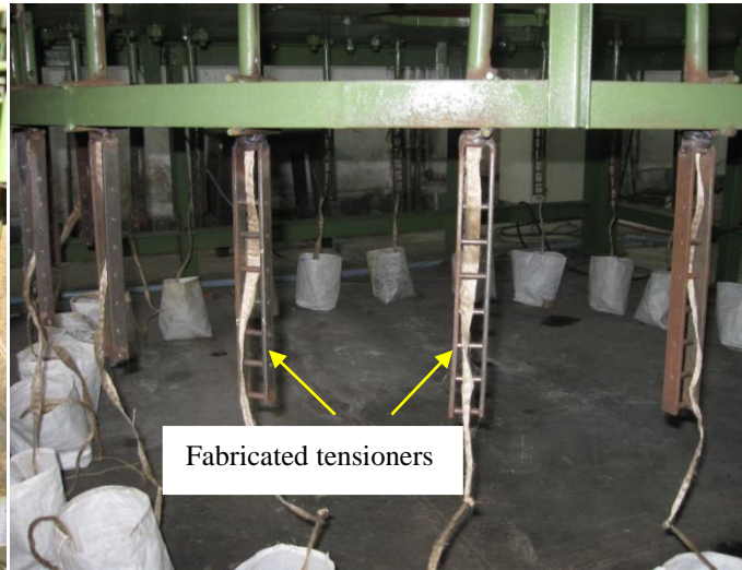
Fig. 6.2.8. Fabricated tensioners for axial materials mounted on the braiding machine
