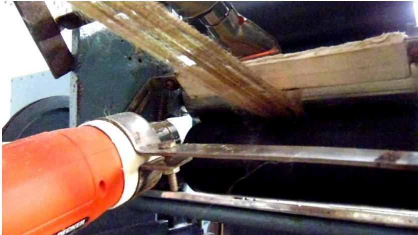
Fig. 9.1.5 Multiple jute tapes coming out of squeezing roller nip and entering drying zone
