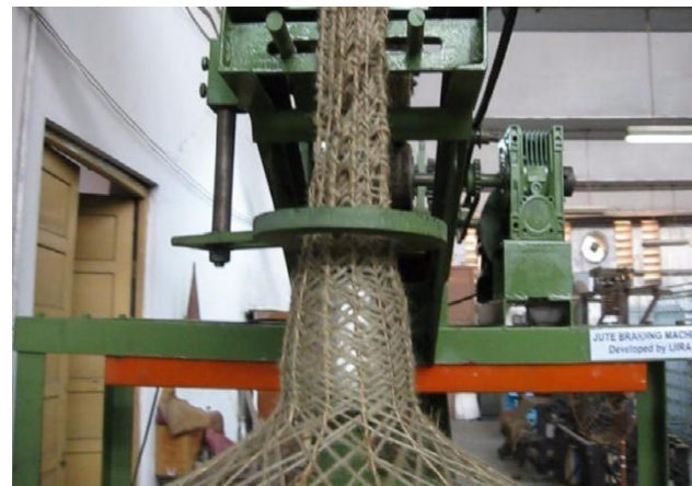
Fig. 6.2.6. Braiding on mandrel
