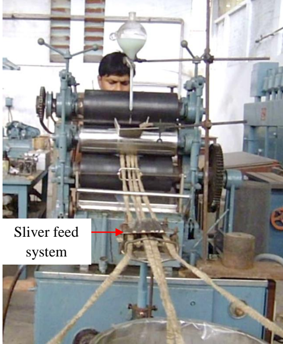
Fig.9.1.1 Front-view of the multiple jute tape preparation model machine
