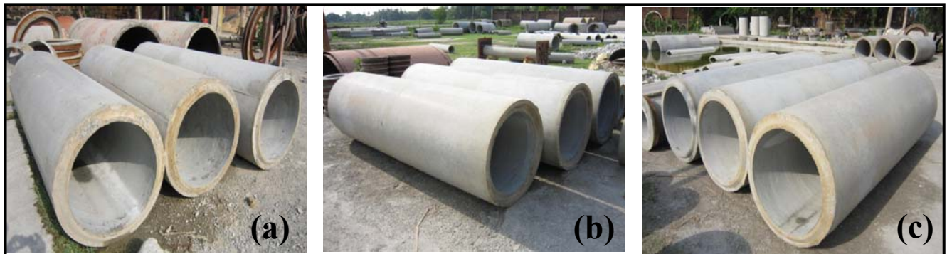
Fig. 15. (a) Pipes without jute fiber reinforcement, (b) pipes with untreated jute fiber reinforcement, (c) pipes with chemically modified jute fiber reinforcement
