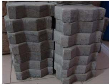
Fig. 21b. Pavers with untreated jute fiber reinforcement
