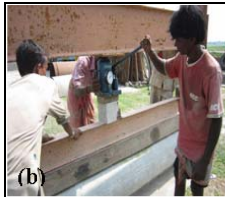
(b) Three edge bearing test of pipes.
