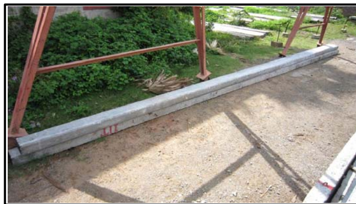
Fig. 18. Chemically modified jute fiber reinforced prestressed concrete pole
