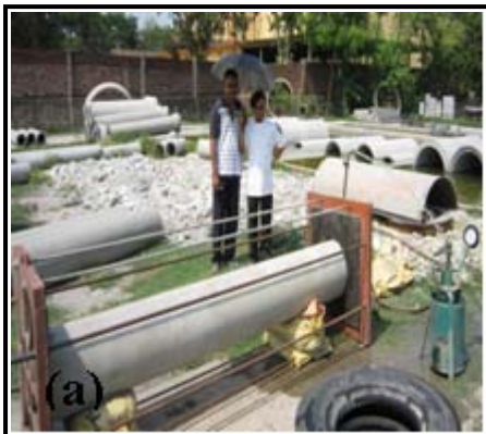
Fig. 16. (a) Hydrostatic testing of pipes,
