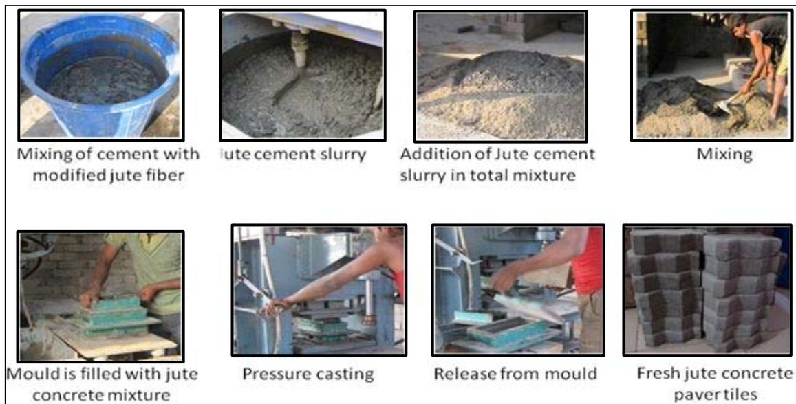
Fig. 20. Fabrication process of chemically modified jute fiber reinforced concrete pavers block
