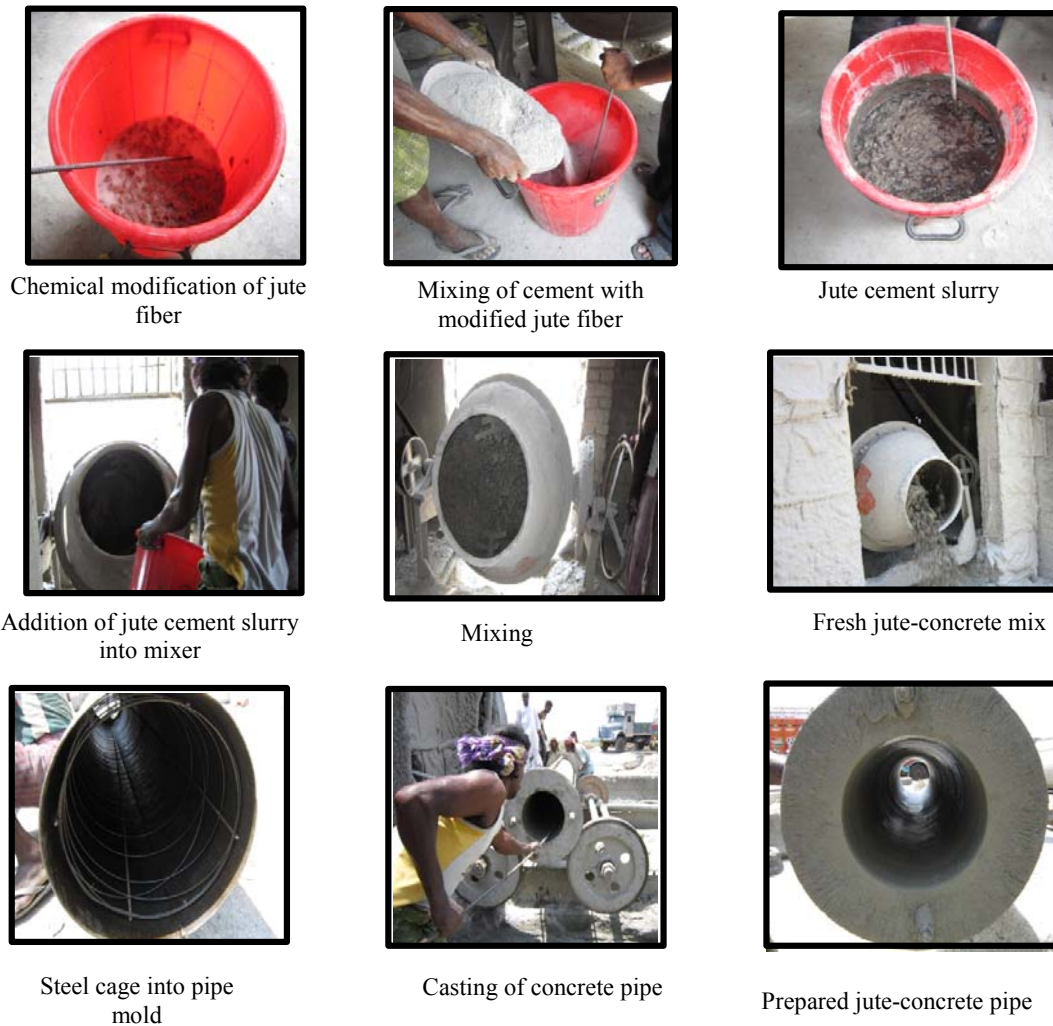
Fig. 14. Fabrication of chemically modified jute fiber reinforced precast concrete pipe
