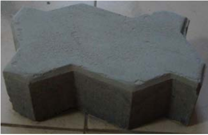
Fig. 21a. Paver without jute fiber reinforcement
