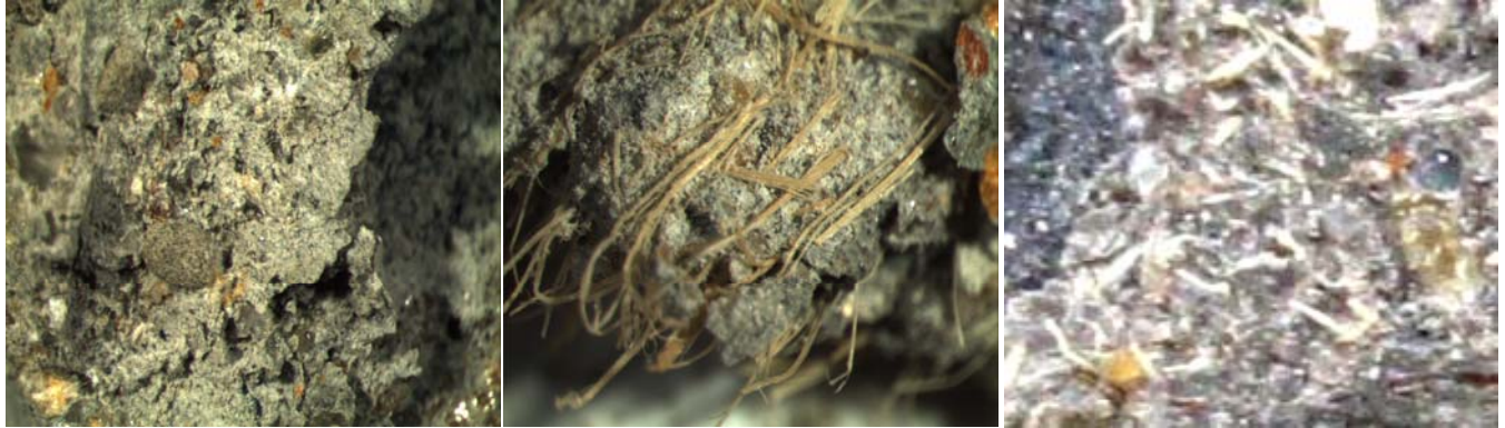
Fig. 13a Microstructure of reference cement concrete
