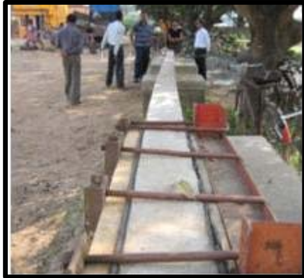
Fig. 19a. Cantilever testing of modified jute fiber reinforced concrete electric pole
