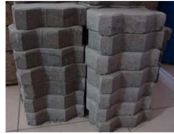
Fig. 21c. Pavers with chemically modified jute fiber reinforcement
