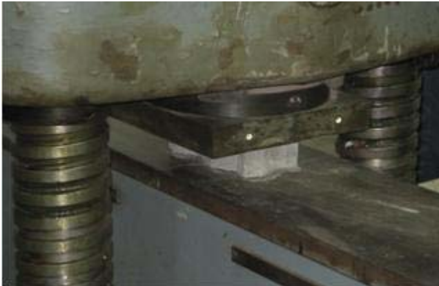
Fig. 22a. Compressive test of jute reinforced concrete paver block
