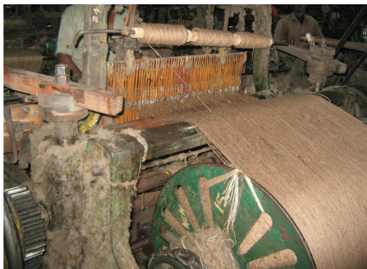
Figure 13. Weaving of FIMG at Kamarhatty Jute Mill
