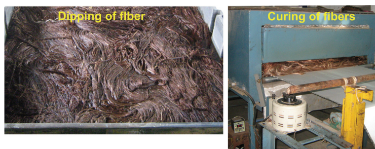
Figure 4. Treatment of jute fibers in KETex
