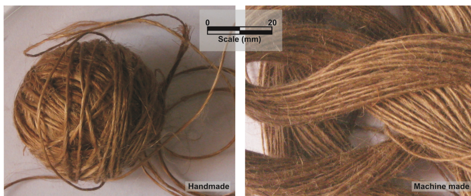
Figure 7. Hand and machine made yarns
