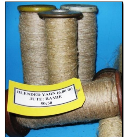
Pic.-15 J-R blended yarn produced in Jute Spg. System
