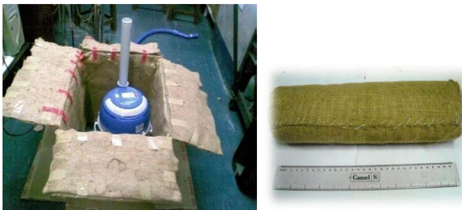
Figure F1: Vacuum cleaner with jute enclosure and jute muffler
