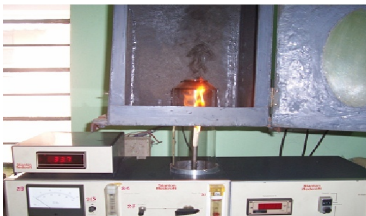
Figure 11: Limiting oxygen index test setup
