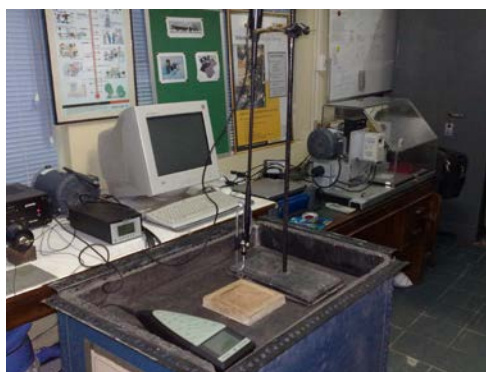
Figure 26: Setup for measurement of transmission loss
