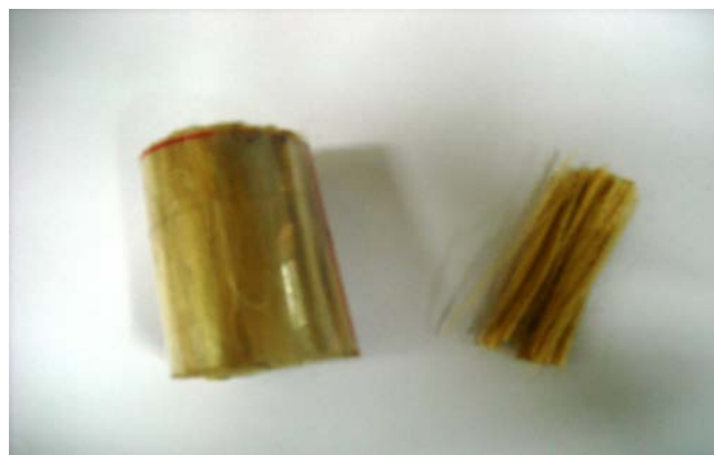
Figure 15: Untreated jute fibre (50 mm x 35 mm \Phi ) sample for measuring its sound absorbing coefficient.
