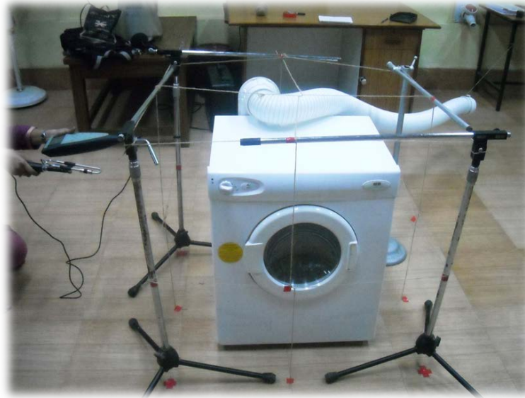
Figure 39: Sound power measurement setup of a domestic dryer
