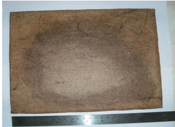
Figure 27: 5% NR latex jute composite, (254 × 254 × 5) mm, (STC-39.5)
