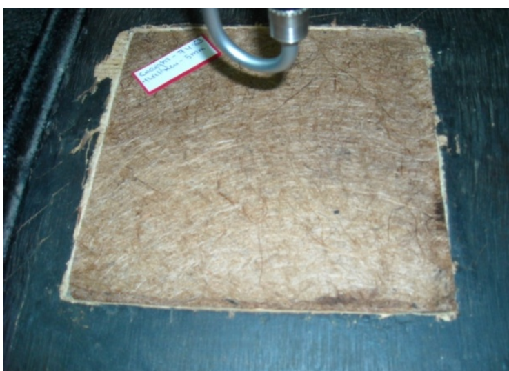
Figure 1: 5% NR Latex Jute Composite
