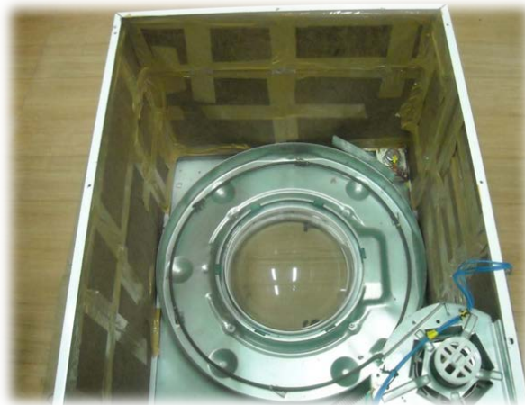
Figure 44: Dryer Shell lined with Jute Composite
