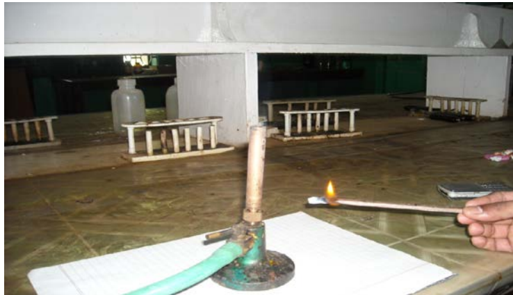
Figure 12: LPG flame propagation of NR latex jute composite.
