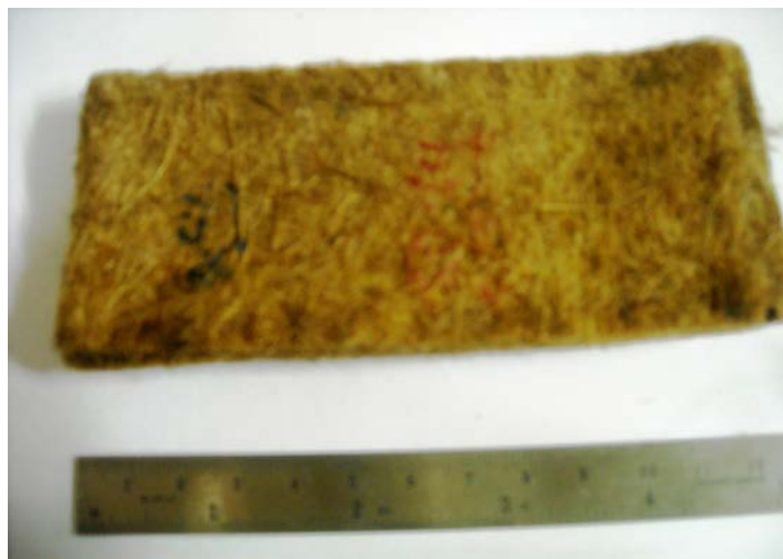
Figure 7: 5% NR latex jute composite after biodegradation test (30 days)
