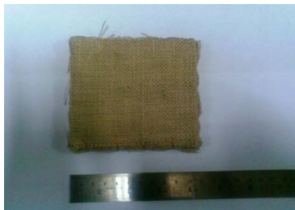
Figure 28: Jute felt+Cloth composite, (152 × 152 × 12.7) mm, (STC-31.8)
