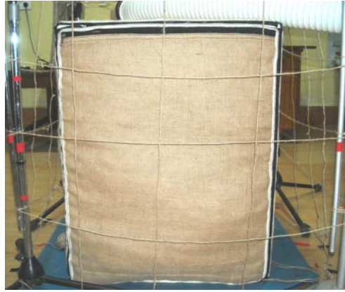
Figure F2: Domestic dryer with jute acoustical blanket
