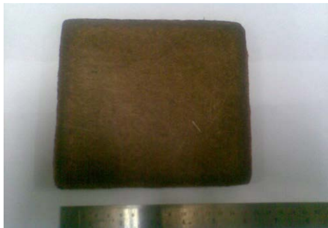
Figure 28: Jute felt+Cloth composite, (152 × 152 × 12.7) mm, (STC-31.8)
